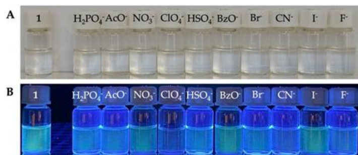
Figure 4. Solutions of compound 1 , in ACN/water (75:25), after adding 50 equivalents of anions, under natural light (A) and UV radiation at 365 nm (B).
