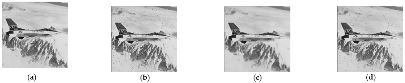
Figure 2. Filtering results for sample image “Airplane”; (a) input image; (b) image with noise added to (a); (c) filtering result of (b) by L2GFI; (d) filtering result of (b) by NLMF.
