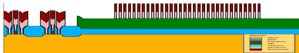
Figure 5. Titanium and aluminum etch.
