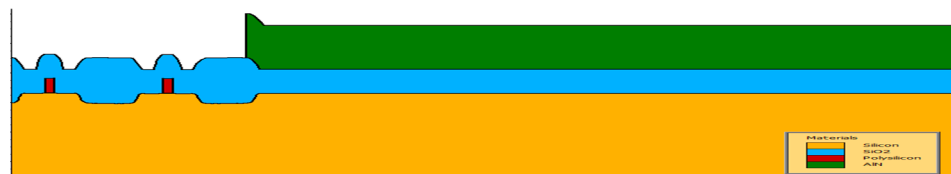
Figure 2. AlN piezoelectric layer deposition.
