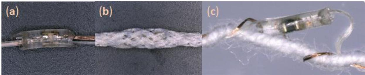
**Figure 1.** Microscope images of E-yarns. (a) The core structure of the E-yarn, including the conductive wire, the soldered component, and the supporting yarn. (b) The final E-yarn. (c) Image showing the failure of the conductive wire at the micro-pod interface after a wash test.
