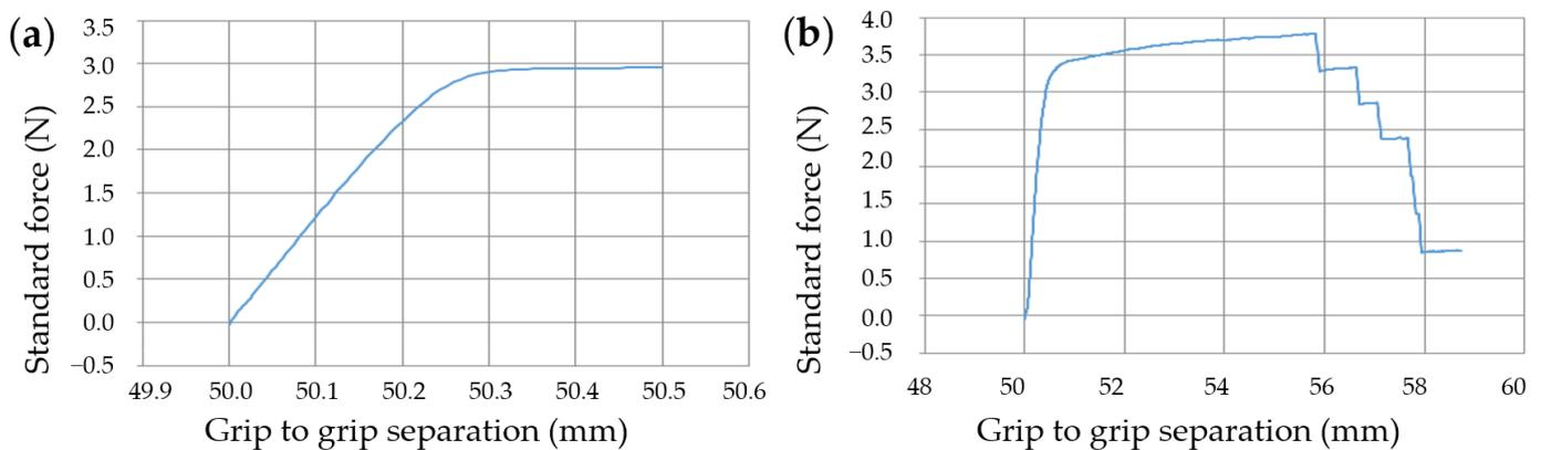
**Figure 2.** Tensile test results of the core structure of the E-yarn: (a) before encapsulation; (b) after encapsulation.
