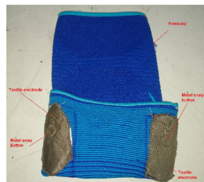
Figure 6. Textile electrode attached to the inside of kneecap.
