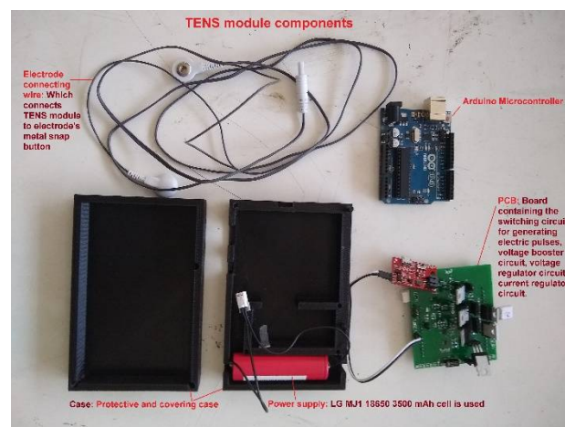
Figure 8. TENS module components.
