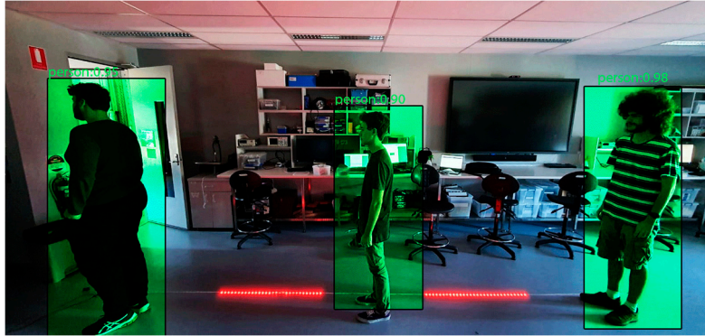
Figure 4. Screenshot of MobileNet-SSD detecting persons using Caffe model in OpenCV.
