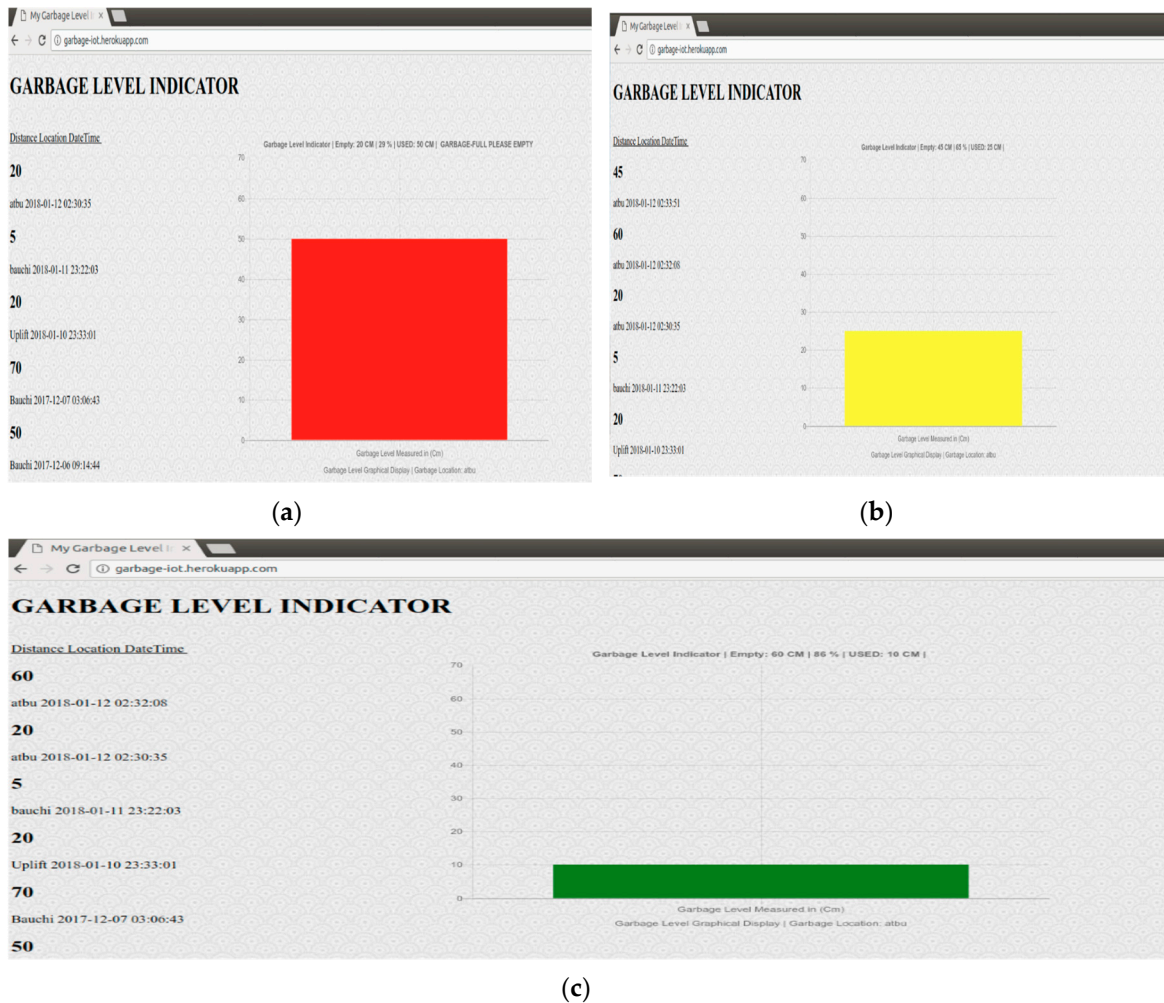
Figure 3. (a) The garbage bin is almost full and is due for collection; the status is “filled”. (b) The garbage bin is half-filled; the status is also “half-filled”. (c) The garbage bin is almost empty; the status is “empty”.
