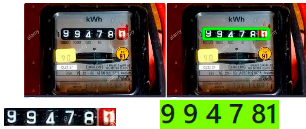
Figure 2. Original image (top left), region of interest that is automatically selected (top right), ROI cropped (bottom left), and digits extracted (bottom right).
