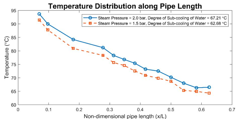
**Figure 3.** Temperature distribution along pipe length for two operating conditions.
