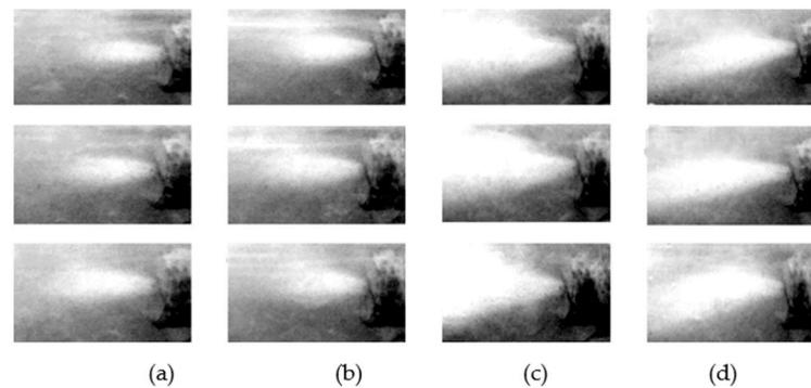
**Figure 2.** Variations in steam plumes with increasing water temperature (plume elongation) at 1.5 bar: (a) conical plumes; (b) elliptical plumes; (c) divergent plumes; (d) plumes with an inclination angle.
