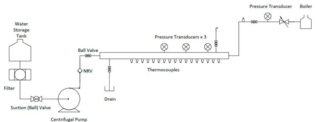
**Figure 1.** Schematic representation of DCC setup.
