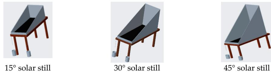
Figure 1. Solar stills with different inclination angles.
