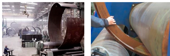
Figure 1. Roll bending machine (left) and result control with templates (right).
