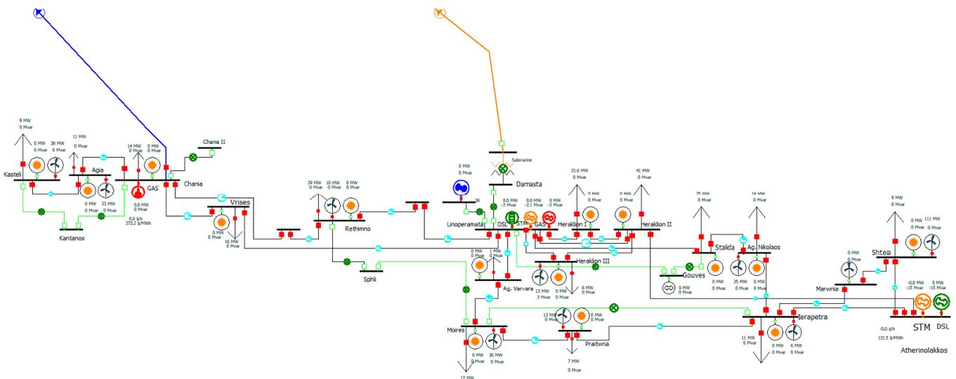
**Figure 6.** Electric grid of Cretan island simulated in Powerworld software.
