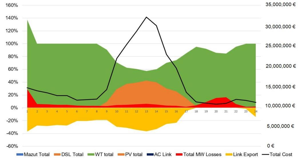
Figure 10. Energy produced on a 24 h basis, including losses and relevant costs in the case of scenario B.
