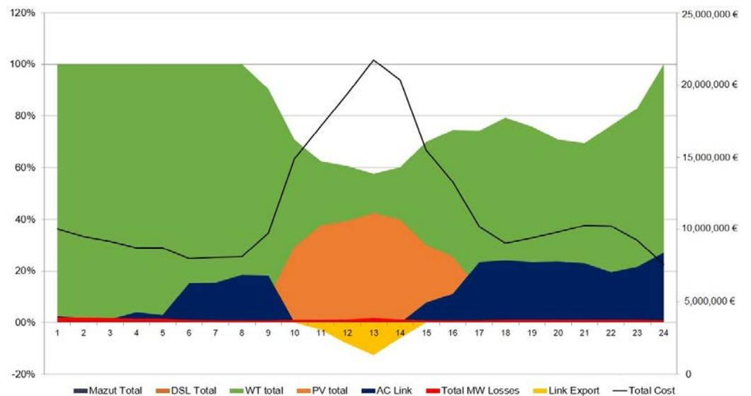
Figure 8. Energy produced on a 24 h basis, including losses and relevant costs in the case of scenario A.
