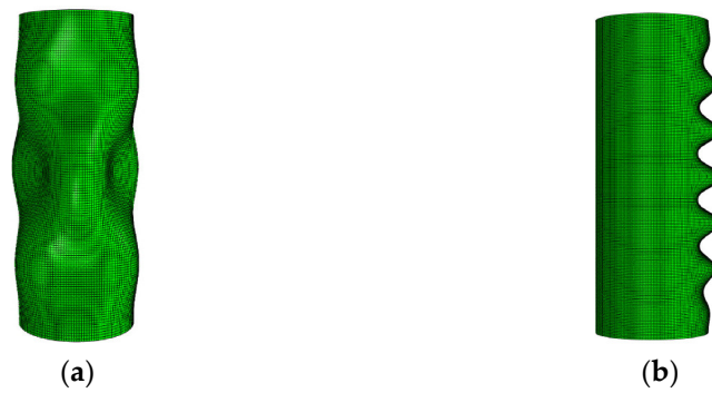
Figure 4. Typical elastic buckling modes (corresponding to lowest eigenvalues). (a) Under axial compression. (b) Under eccentric compression or pure bending.
