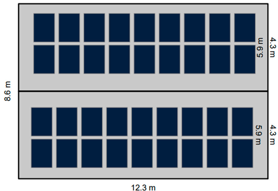
Figure 2. Top-view of the solar panels' placements.
