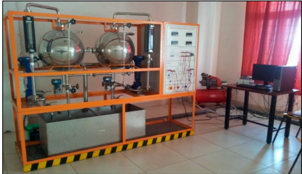
Figure 1. Real-time experimental setup of the DITS liquid level process.
