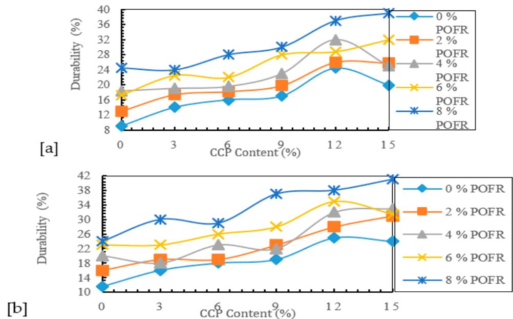
Figure 4. Durability of (a) BCS-CCP-POFR and (b) RLS-CCP-POFR.
