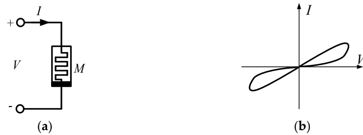
Figure 3. Memristor [7]: (a) symbol; (b) I - V characteristic curve.
