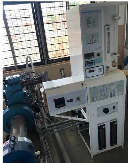
Figure 1. Setup of CRDI Engine.
