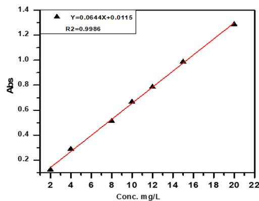
**Figure 1.** Calibration curve of methylene blue dye.
