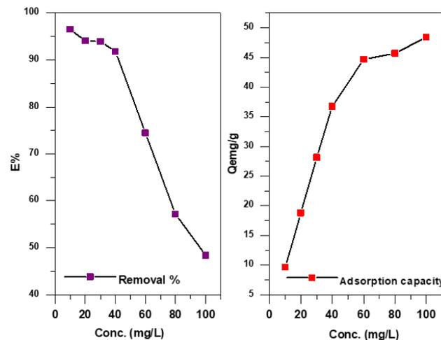
**Figure 5.** Effect of various concentrations of methylene blue dye on removal percentage and adsorption capacity.
