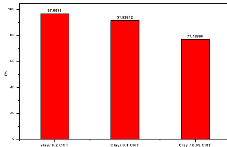
**Figure 8.** Comparative study among 0.2 g carbon nanotube (CNT)/clay (bentonite), 0.1 g CNT/clay, and 0.05 g CNT/clay surfaces as adsorbents for methylene blue dye removal.
