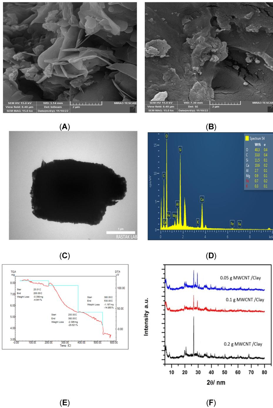
**Figure 3.** Field emission scanning electron microscopy (FESEM) image of multi-walled carbon nanotube (MWCNT)/clay (bentonite) (A) before and (B) after adsorption. (C) Transmission electron microscopy (TEM) image of MWCNT/clay. (D) Energy-dispersive X-ray (EDX) spectroscopy image of MWCNT/clay. (E) Thermogravimetric analysis (TGA) image of MWCNT/clay. (F) X-ray diffraction (XRD) image of MWCNT/clay.
