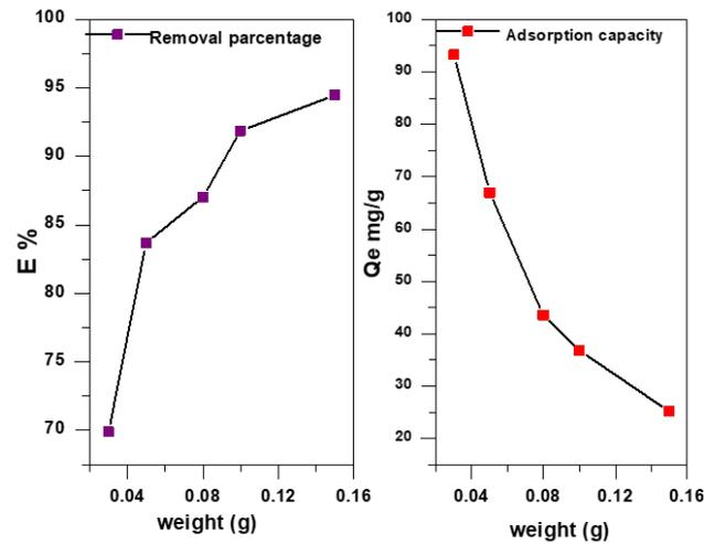
**Figure 4.** Effect of the weight of multi-walled carbon nanotube (MWCNT)/clay nanocomposites on the surface.
