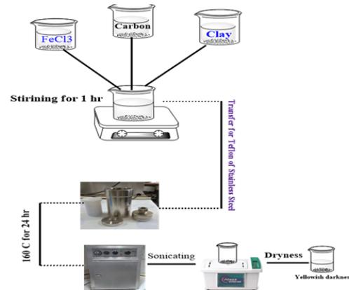
**Figure 2.** Preparation of multi-walled carbon nanotube (MWCNT)/clay (bentonite) nanocomposite.
