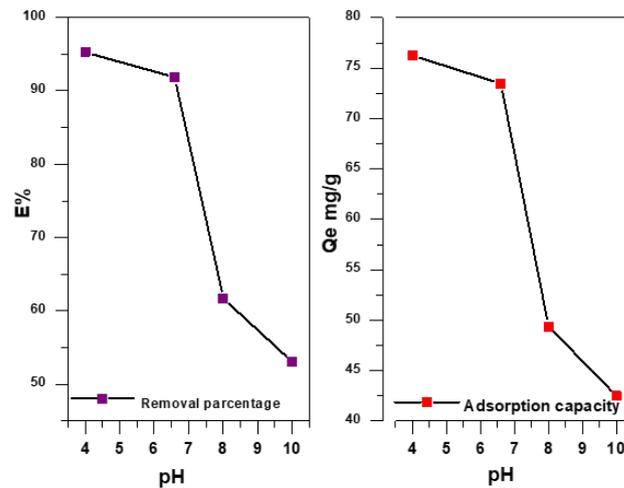
**Figure 7.** Effect of solution pH on the adsorption of methylene blue dye using multi-walled carbon nanotube (MWCNT)/clay nanocomposites.
