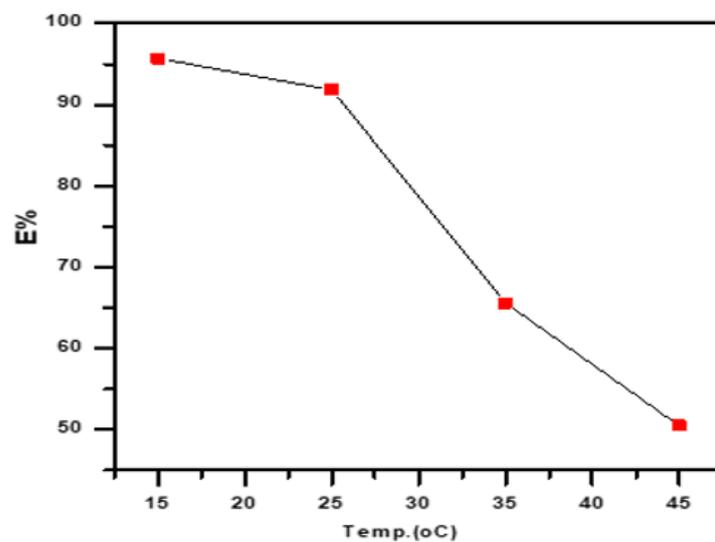
**Figure 6.** Effect of solution temperature on the removal efficiency of multi-walled carbon nanotube (MWCNT)/clay nanocomposites for methylene blue dye.
