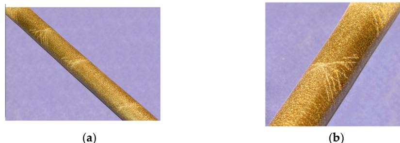
**Figure 1.** Luder's band. (a) Cluster of Luder's band. (b) Closed-up look on one of the clusters [1].
