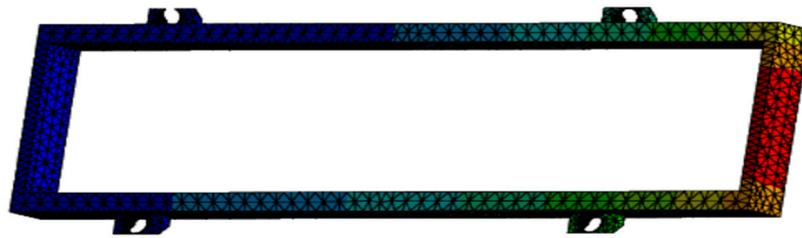
**Figure 7.** Thermal analysis for Inconel-718 subjected to the boundary conditions specified in Table 3.
