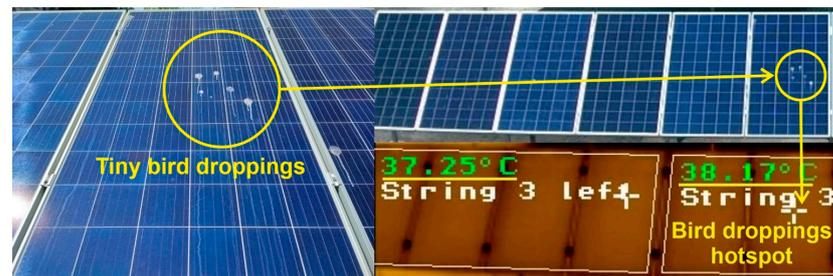
**Figure 3.** Example for several thin bird droppings and the resulting hotspot.
