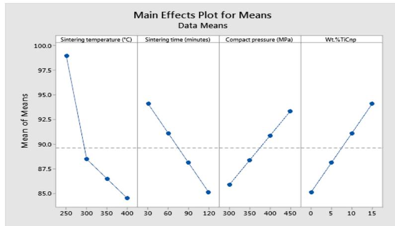
Figure 1. Main effect plot for means of microhardness.
