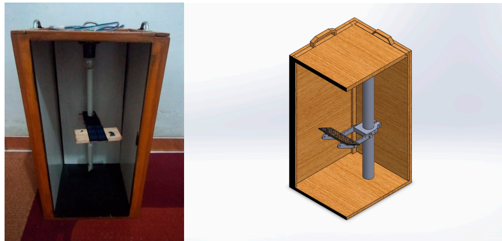
Figure 1. Indoor photovoltaic test tool.
