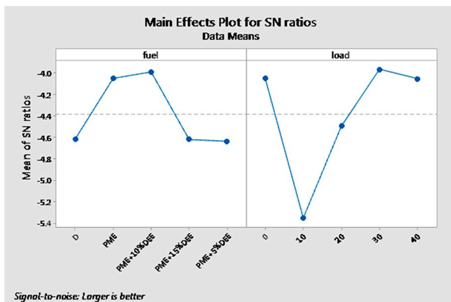
Figure 3. Main effect plots for signal-to-noise ratio for fuel blend and load.
