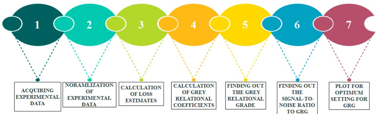
Figure 2. Schematic diagram of gray relational analysis.
