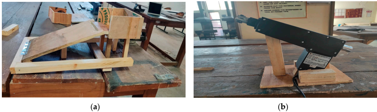
Figure 4. (a) Side view of ramp with trolley. (b) Side view of actuator mounted on the table.
