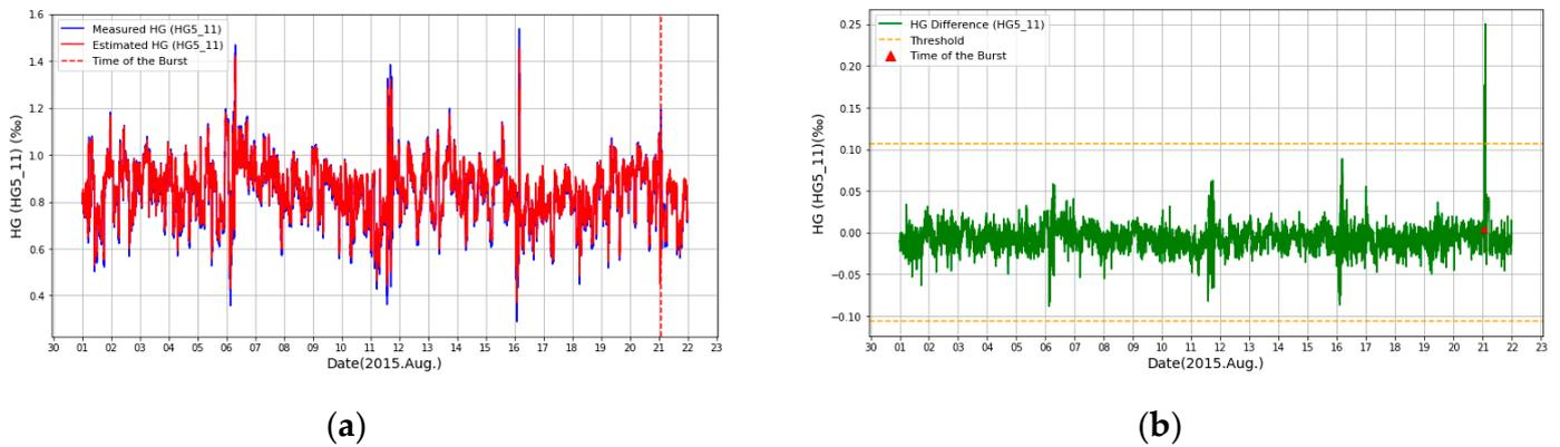
Figure 2. Hydraulic gradient changes in the model ( $HG_{5,11}$ ): (a) Measured HG and estimated HG in the model; (b) HG difference and threshold in the model.
