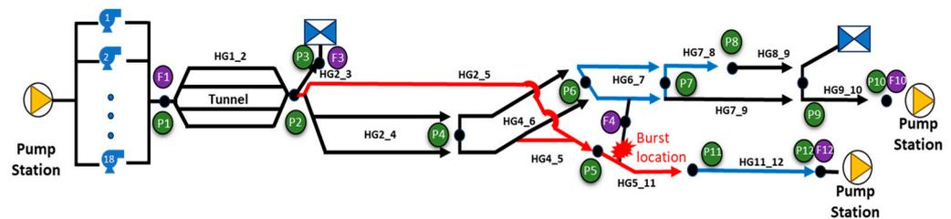
Figure 4. HG<sub>diff</sub> map for the burst localization.
