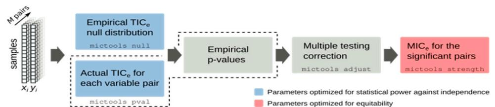
Figure 1. The MIC technique pipeline.
