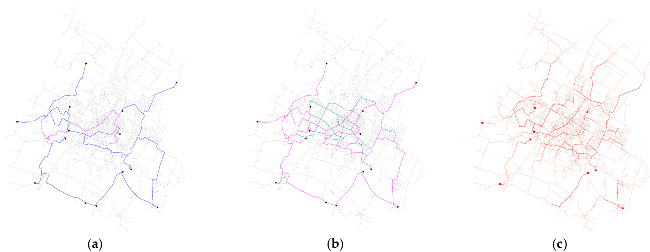
Figure 1. Primary Networks for Emilia Network—(a) in blue the Steiner tree by T1, in magenta the added shortest paths edges by T2 ( k = 1 ) (b) in teal the added k -shortest paths edges T2 ( k > 1 ); (c) in dark red Consumption approach results by T3 as presented in Table 1.
