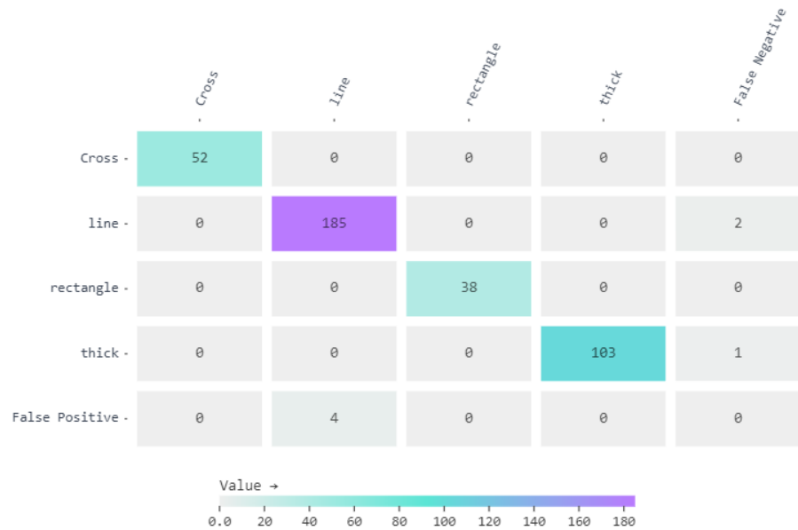
Figure 5. Confusion matrix evaluated at 0.2 confidence threshold on validation and test datasets, leading to a precision of 93% and a recall of 99%.
