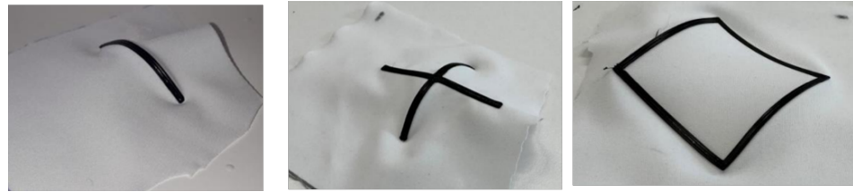
Figure 2. Exemplary geometries of the 3D printed stiffeners.
