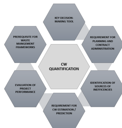
Figure 1. Functions of CW quantification in construction management.
