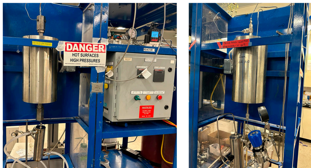
Figure 5. Laboratory-scale packed-bed reactors employed in the generation of hydrogen from different hydrocarbons.
