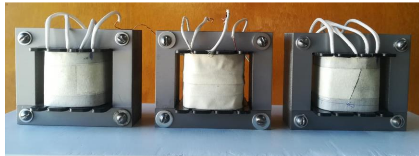
Figure 4. Single-phase inductor bank for an inductive compensation module: 53 VAR, 220 V, 1.5914 H, 1.0609 H and 0.7957 H, respectively.
