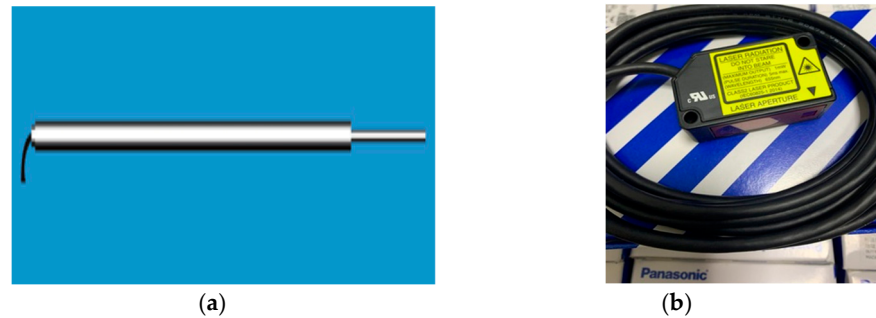
Figure 2. Adopted displacement sensors: (a) Keyu LVDT-WYDC contact displacement sensor; (b) Panasonic HG-C1030 laser displacement sensor.
