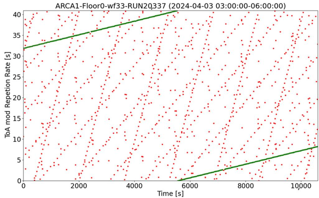
**Figure 4.** Modulus between the selected ToAs and the RR plotted as a function of time. This example illustrates the APS data from the ARCA hydrophone in DU1 related to WF33.
