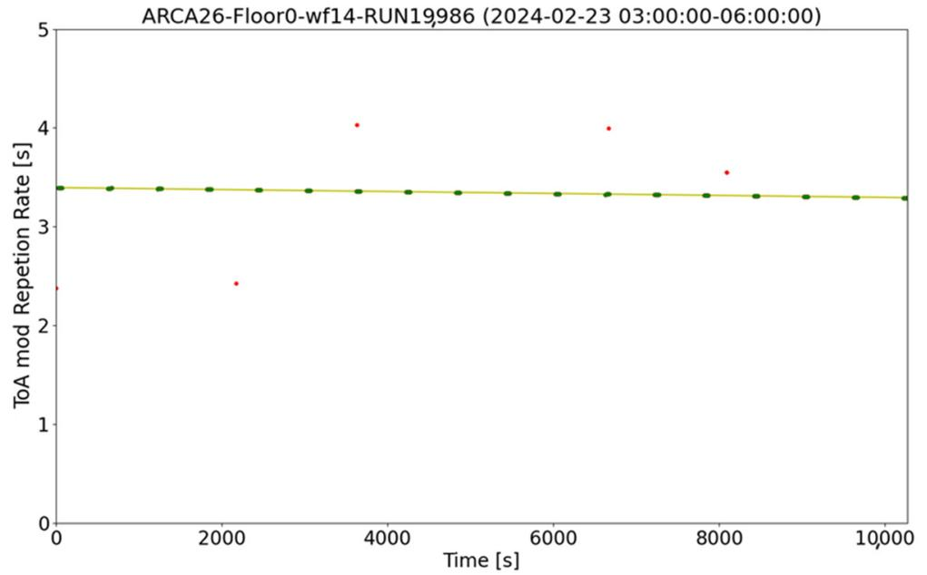
**Figure 3.** Modulus between the selected ToAs and the RR plotted as a function of time. The correct ToAs (highlighted in green) align along a straight line. This example illustrates the APS data from the ARCA hydrophone in DU26 related to WF14.
