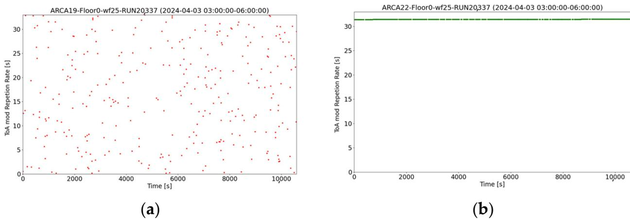
**Figure 6.** Modulus of the selected ToAs and the RR plotted as a function of time. **(a)** Incorrect ToAs. Data from the ARCA hydrophone in DU19, where ToAs deviate from the expected alignment, suggesting a potential issue with this hydrophone. **(b)** Correct ToAs. Data from the ARCA hydrophone in DU22, where ToAs align correctly along the expected straight line, indicating proper functioning of the AB.
