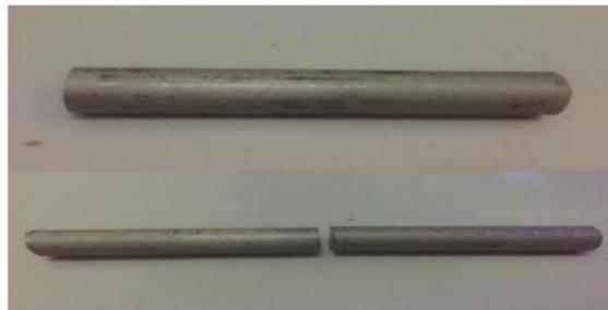
**Figure 1.** The A6061 material for friction welding.
