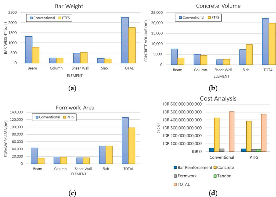
**Figure 4.** Comparison of conventional structures' and PTFS structures' (a) bar weight; (b) concrete volume; (c) formwork area; and (d) overall cost analysis.
