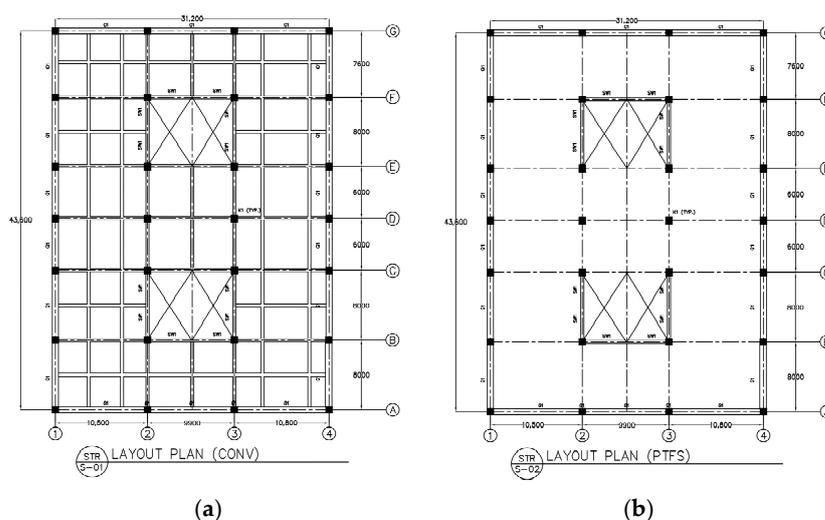
Figure 1. Floor plan: (a) Conventional structure and (b) PTFS structure.
