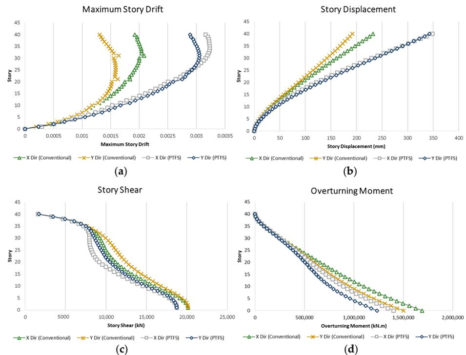
**Figure 3.** Structural responses of conventional and PTFS structures: (a) maximum story drift; (b) story displacement; (c) story shear; and (d) overturning moment.
