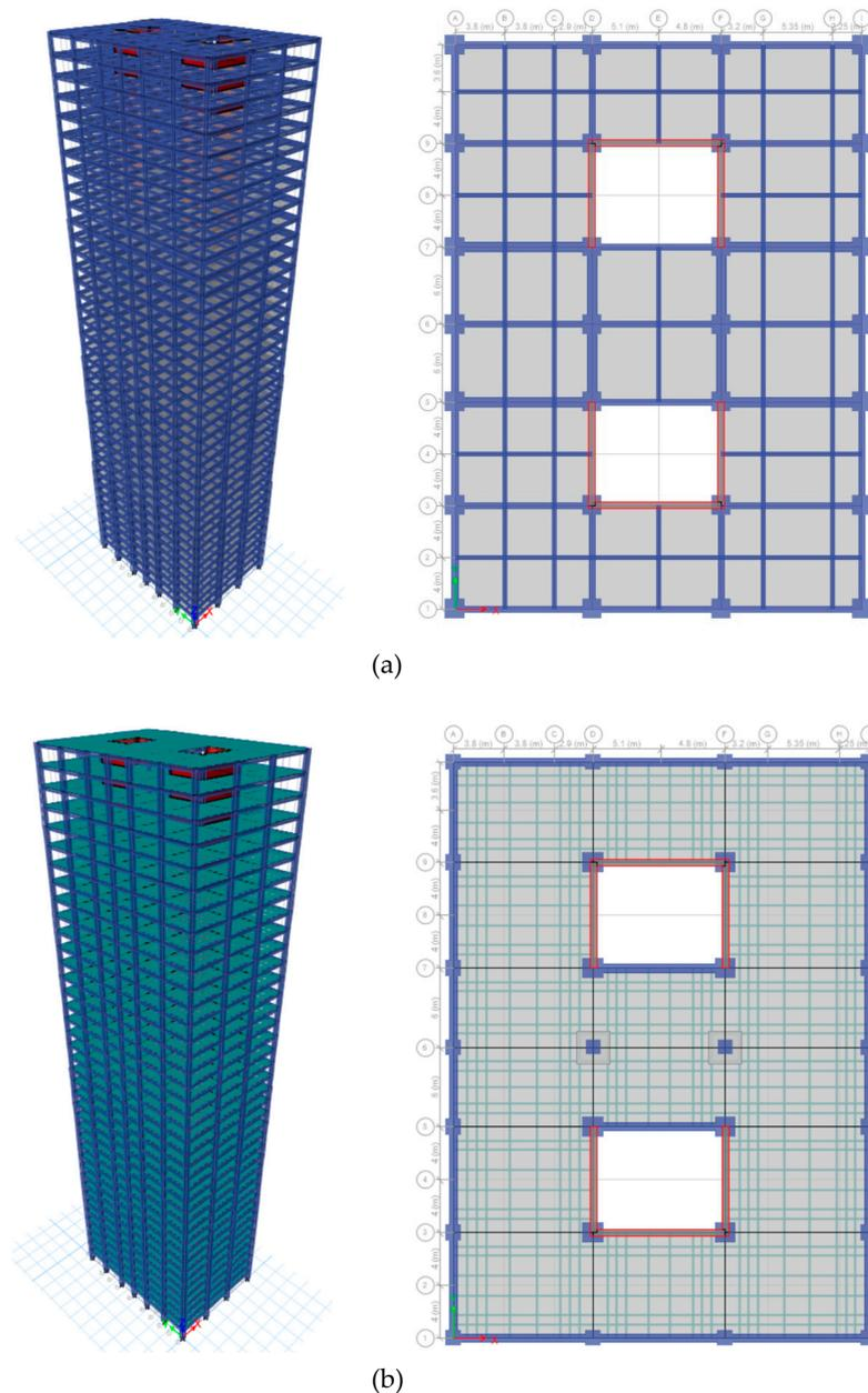
**Figure 2.** ETABS model: (a) Conventional structure and (b) PTFS structure.
