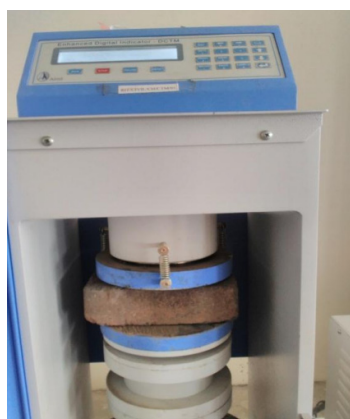
Figure 4. Compressive strength testing of samples.
