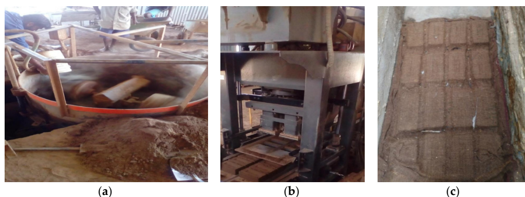
Figure 2. Specimen preparation process: (a) mixing of materials, (b) casting of bricks, and (c) curing of bricks.
