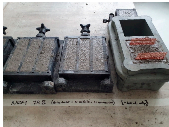
Figure 4. RMCF1 mortar samples.
