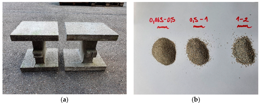
Figure 3. (a) H-shape structural formwork, (b) fractions of waste aggregates.
