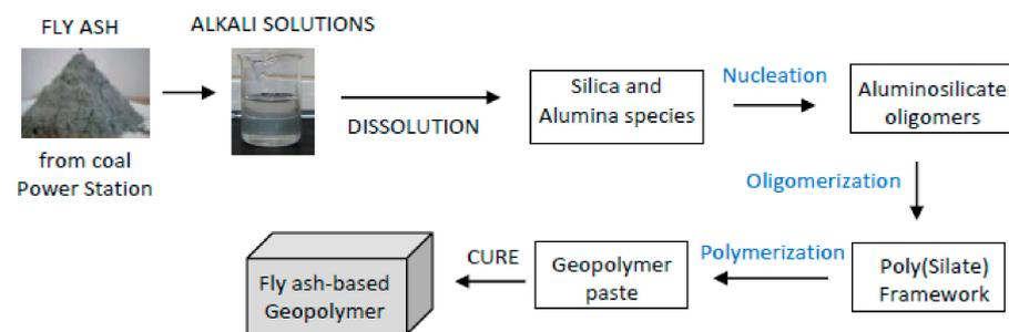
**Figure 1.** The transformation process of fly ash into a binder for geopolymer materials [10,11].
