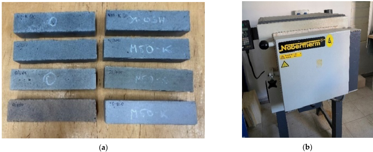
Figure 1. (a) Samples after being heated and cooled down, (b) Electric Furnace NABETHERM.
