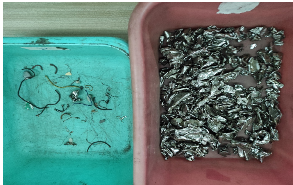
Image 2. Magnetic product from Sample 2 with the blade tilt set at 30°—the left basket contains the contamination of magnetic product and the right one contains the stainless steel pieces.
