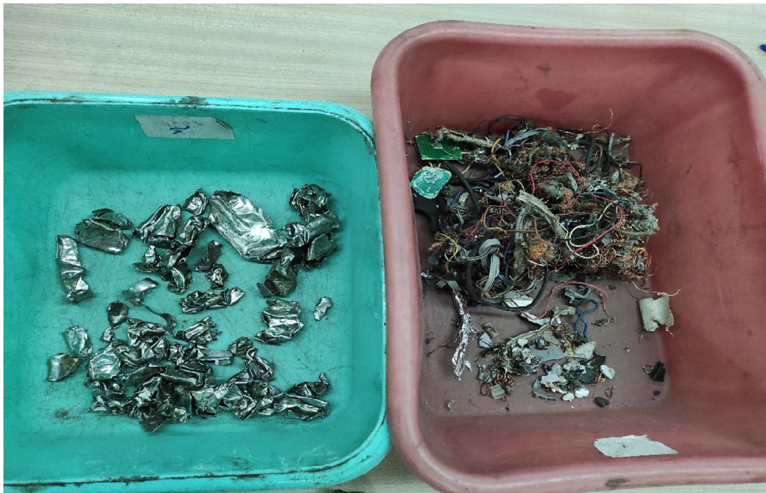
Image 3. The non-magnetic product of Sample 3, with the blade tilt set at 50°—the left basket contains the stainless steel pieces that could not be held and were rejected as the non-magnetic product, while the right basket contains the non-magnetic product.
