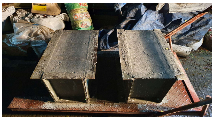
Figure 1. Concrete specimens after pouring and vibration.
