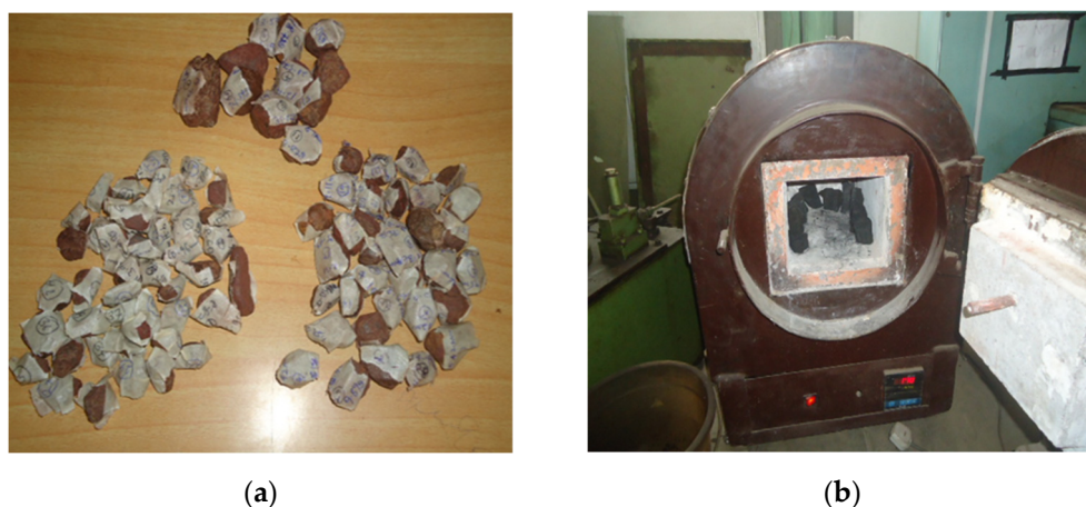
Figure 1. (a) Goethite iron ore samples prepared at different size ranges; (b) the reactor: activated carbon furnace [24].
