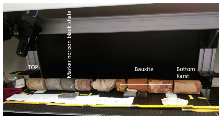
Figure 1. LIBS measurement configuration of composite bauxite profile.
