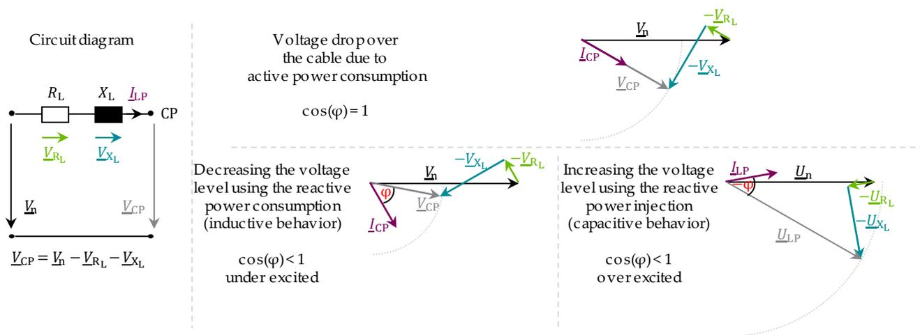
**Figure 7.** The principal operation of reactive power management based on [59].
