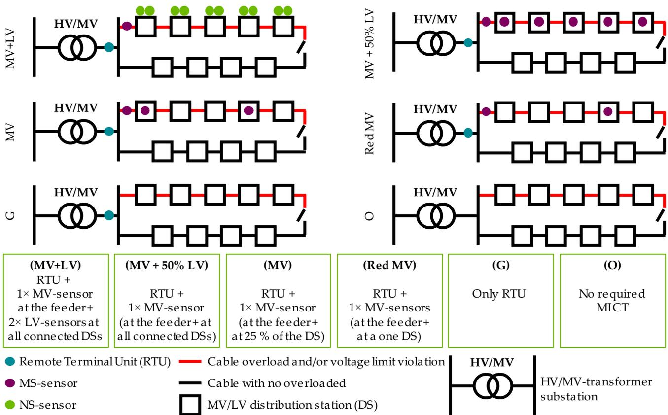
Figure 6. Illustration of the six load management layouts for one medium voltage ring based on [59].
