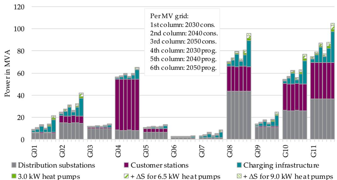
**Figure 8.** Load development for eleven medium voltage grids for the two development scenarios over the years 2030, 2040 and 2050 based on [59].
