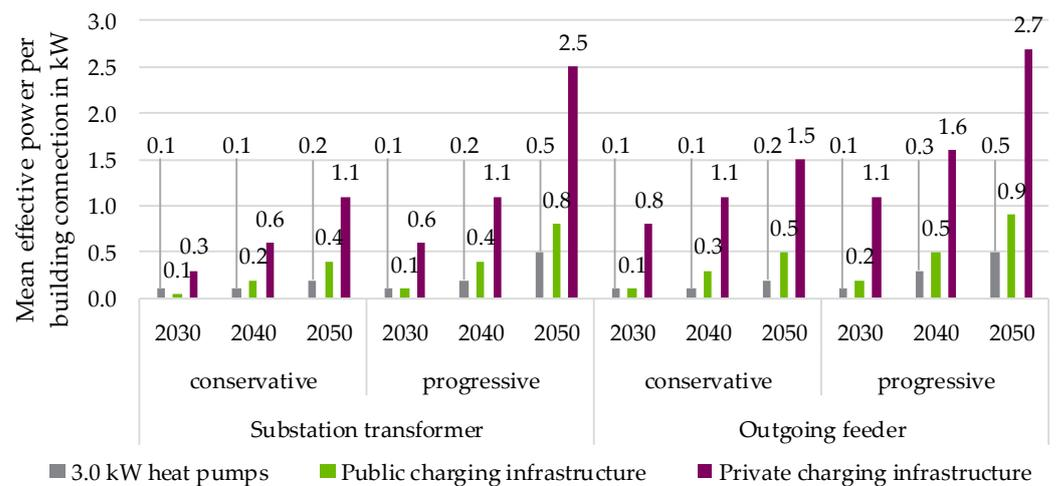
**Figure 12.** Mean effective power per building connection for dimensioning the substation transformer and outgoing feeders for private and public charging infrastructure and 3.0 kW heat pumps.
