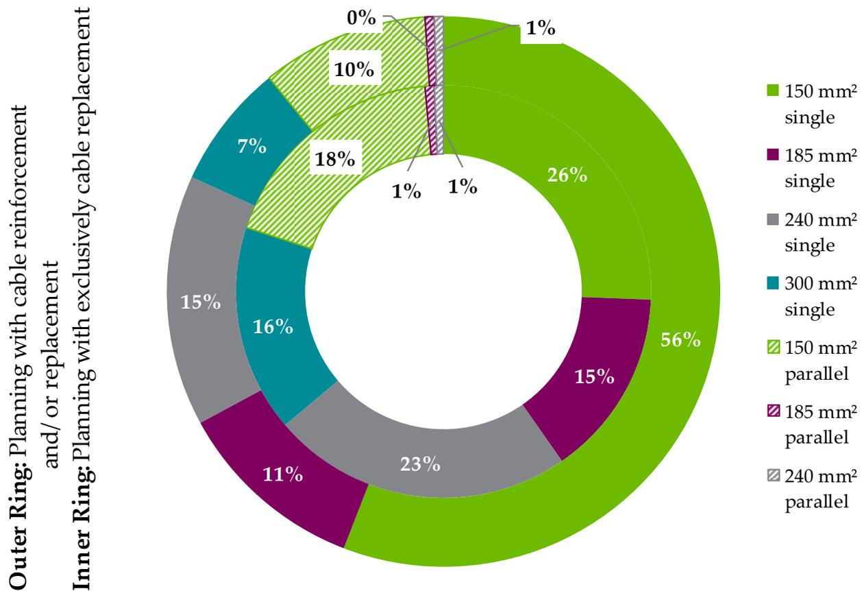
**Figure 14.** Share of cable measures for different cable cross-sections in relation to total cable measures for two planning techniques in the 10 kV grids.
