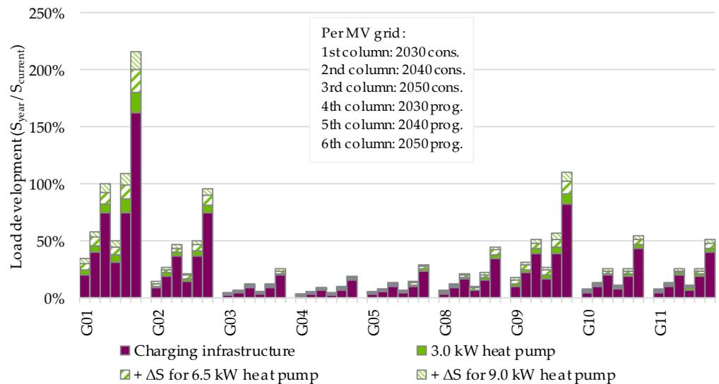
**Figure 15.** Load development for the two development scenarios and the years 2030, 2040, and 2050 in relation to the current load power based on [59].
