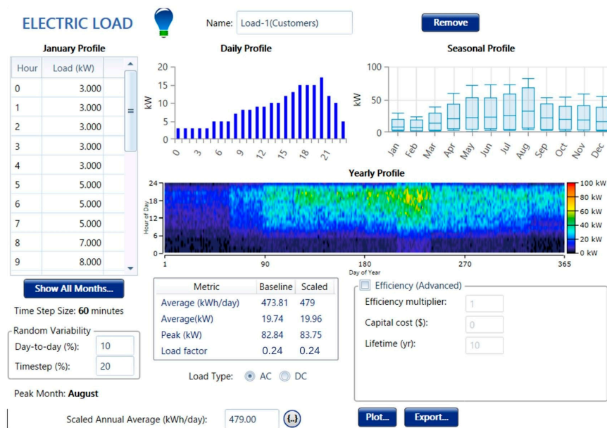
Figure 3. Electrical load data for Load-1.
