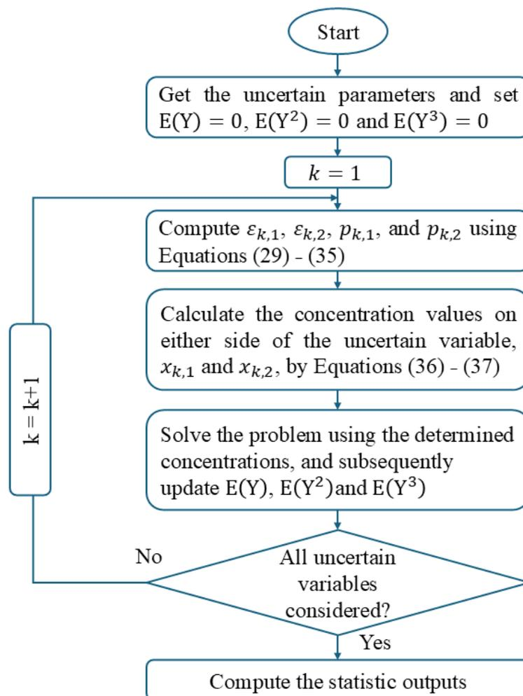
Figure 2. The flowchart of the proposed method.
