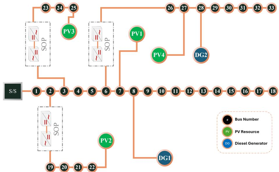
Figure 4. Interconnected multi-microgrids through SOPs (Case 2).
