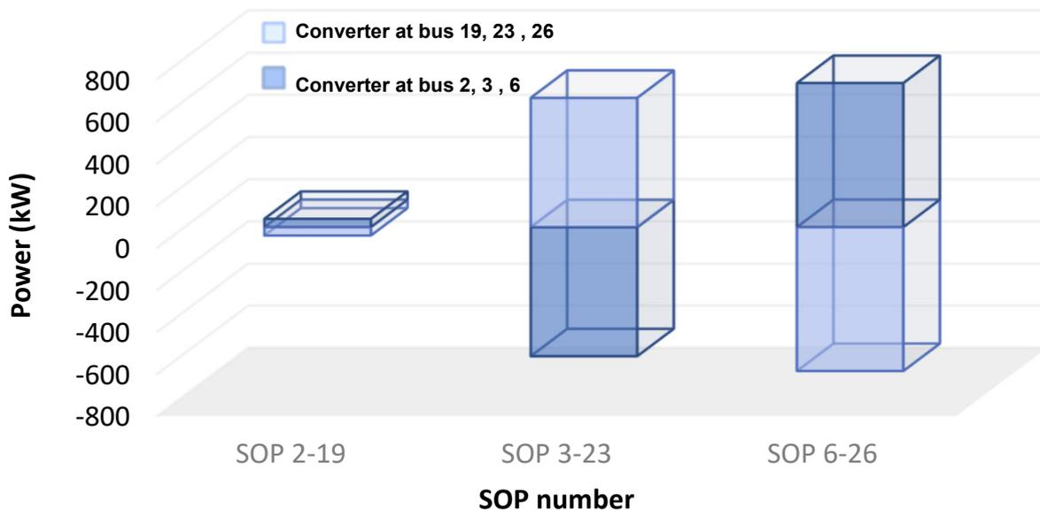
**Figure 8.** Active power transaction among microgrids by SOPs.
