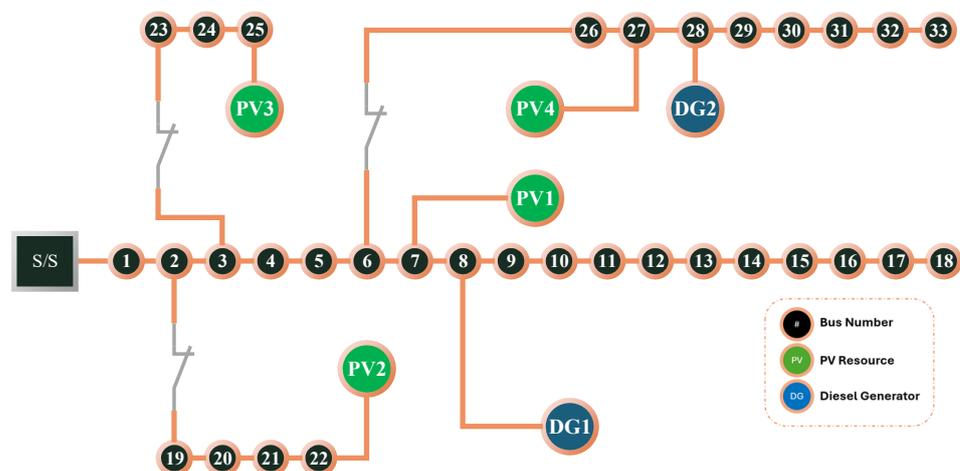
**Figure 3.** Interconnected multi-microgrids with switches (Case 1).
