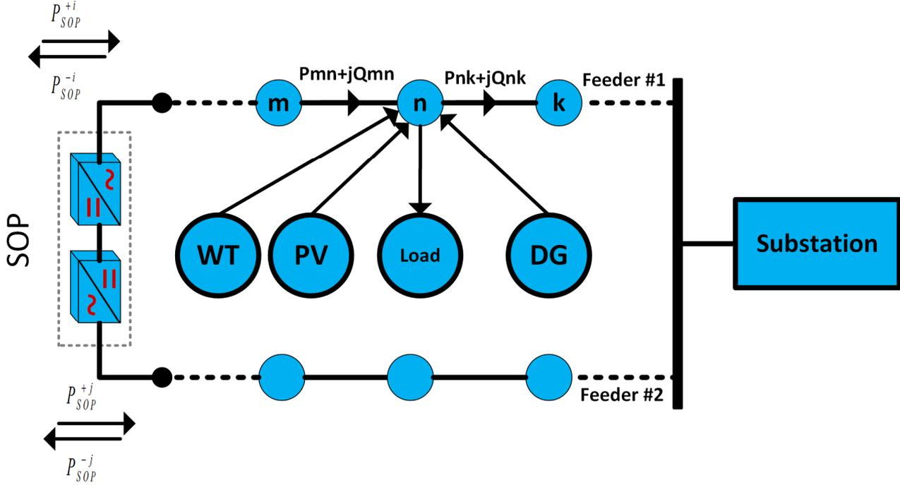
Figure 1. The SOP configuration on a sample network.
