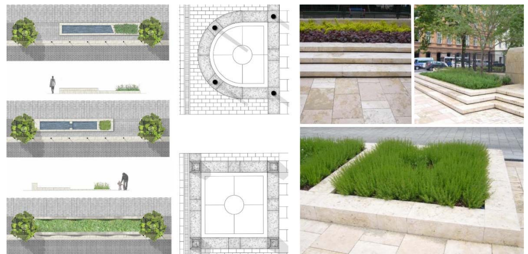
Figure 3. The limited space available and the narrow streets required several elaborate design details for the location of water features and plants. (Photos by the authors, 2012).
