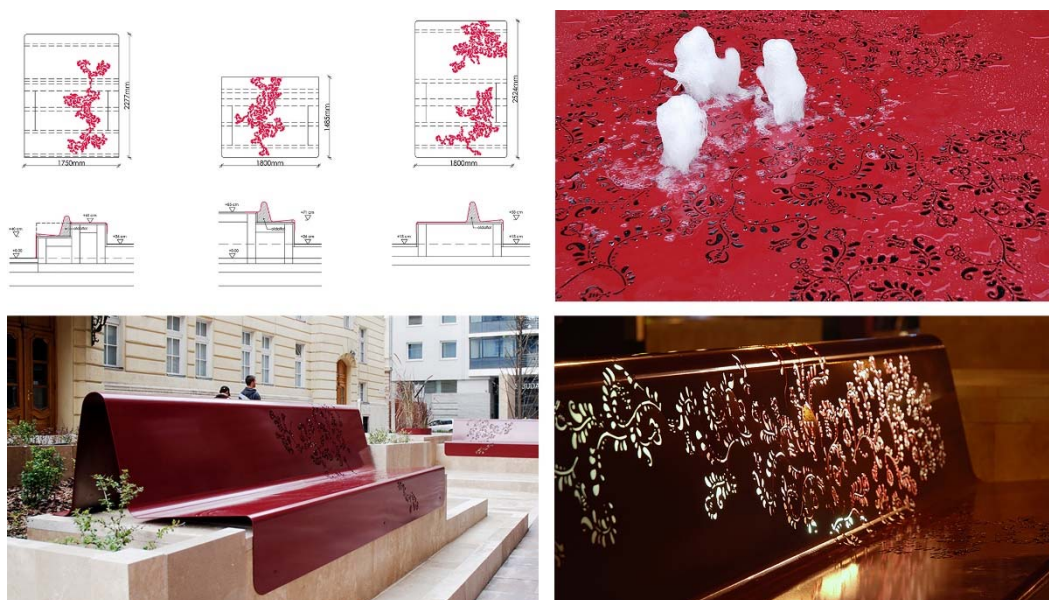
Figure 7. Design detail plans and realised elements of the unique street furniture in the Ditrói Mór street, Budapest. The unique street furniture with innovative design has multiple roles: serving as benches, and also for water features and lighting. The red steel provides a strong contrast to the white limestone slabs that are usual at Budapest public spaces, and thus a characteristic, unique design is achieved at the promenade. (Photos by authors, 2014).
