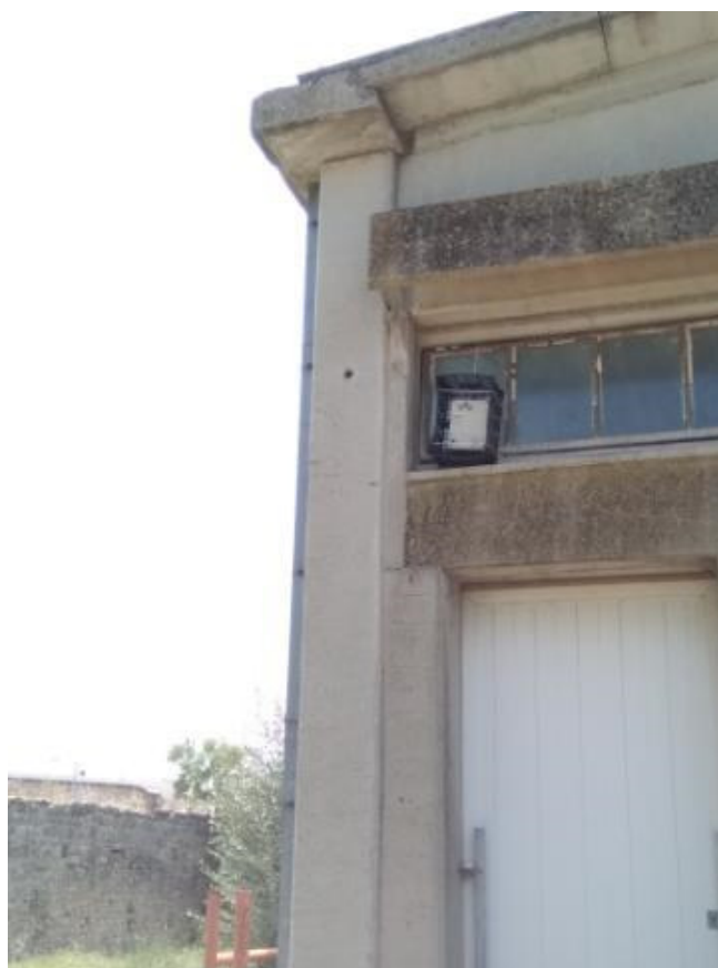
Figure 3. The spot where the second monitoring unit was placed to monitor the air outside the depot. It is located near the depot roof.
