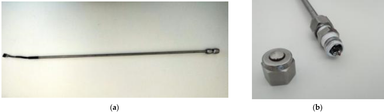
Figure 7. (a) The probe designed and implemented for measuring the temperature inside the manure heaps, which is 1 m long; (b) TC1047A sensor arranged inside the probe head.
