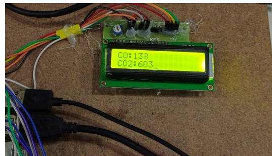
Figure 3. Photograph of the LCD screen showing CO and CO 2 values.
