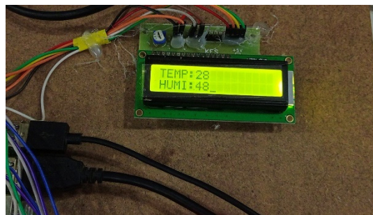
Figure 2. Photograph of the LCD screen showing real-time temperature and humidity readings.
